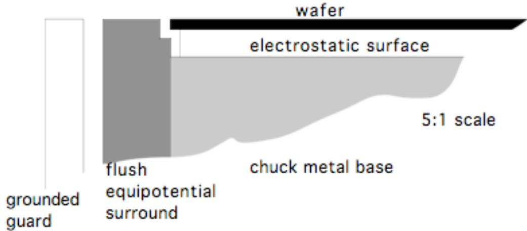
Field plot (-200V bias on wafer, +20V plasma potential with respect to grounded guard)
