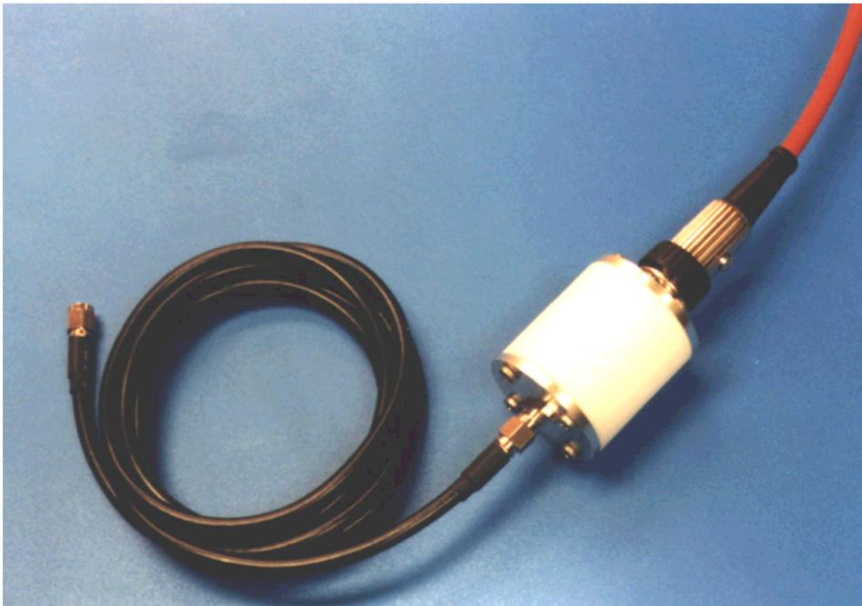
Figure 3. BD5 coupler for rf applications.
