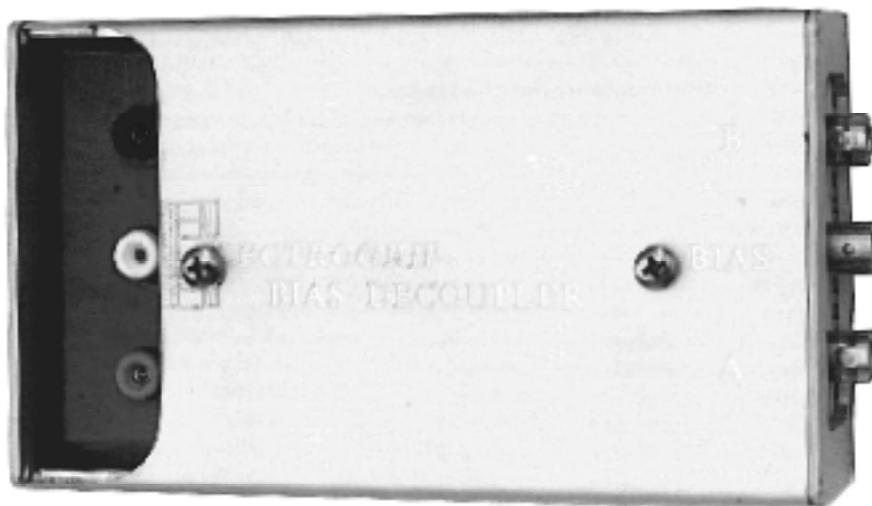
Fig. 1 Bias Decoupler. View of mounting side facing rf enclosure.
